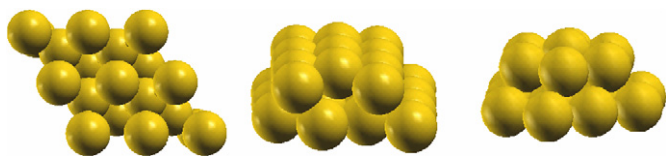
Fig. 1. Schematic representation of gold models: Au(111) (left), Au rod (center), and Au 19 (right).
